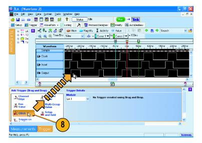
Select the groups that you want the logic analyzer to trigger on. Clear any other channels.
