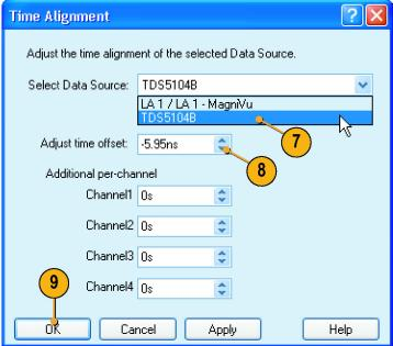
The oscilloscope data is now time-aligned with the logic analyzer data.
