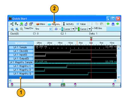
3. Click the Zoom Out button until you see the entire MagniVu timing waveforms. Note that the MagniVu timing data is 16 K bits long as compared to the Deep timing data. Deep timing lets you acquire a large amount of data; MagniVu timing lets you focus on the details of the data.
