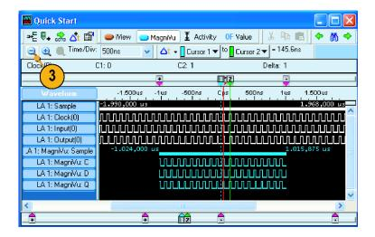
Move Cursor 1 to an area in the Waveform window outside the range of the MagniVu data.
