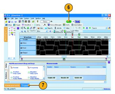
Click and drag the Glitch icon from the Tabbed Trigger window to the Output group waveform.
