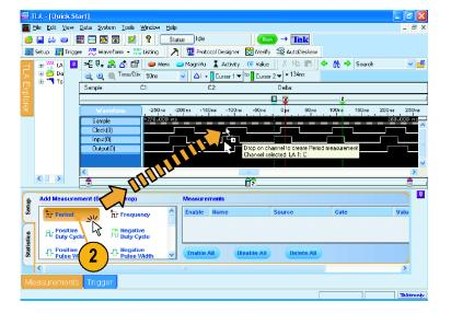
4. Click the Statistics tab in the Data Measurement window to display the results of the measurement along with other statistics. Measurements are taken on the existing data without having to acquire new data.
