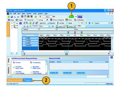
3. Click and drag the **Channel Edge** icon from the Tabbed Trigger window to the Output waveform (channel).
