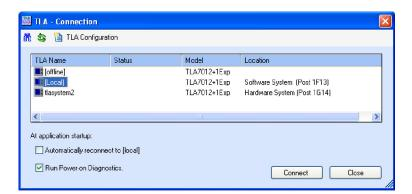
Connect as Remote Host when you want to run the application on your PC to control the instrument remotely, and then store the data locally on your PC.
