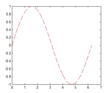
The 'r--' string is a *line specification*. Each specification can include characters for the line color, style, and marker. A marker is a symbol that appears at each plotted data point, such as a +, o, or \*. For example, 'g:\*' requests a dotted green line with \* markers.
