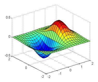
Both the surf function and its companion mesh display surfaces in three dimensions. surf displays both the connecting lines and the faces of the surface in color. mesh produces wireframe surfaces that color only the lines connecting the defining points.
