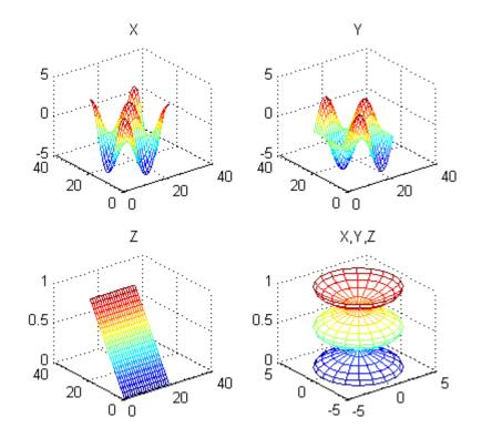
The first two inputs to the subplot function indicate the number of plots in each row and column. The third input specifies which plot is active.
